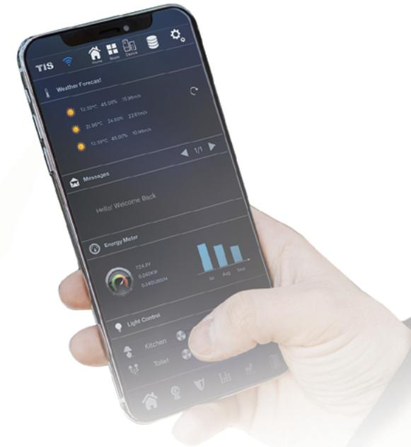
If monthly consumption, for example, reaches or passes the standard tier's maximum limit (overusage is shown by red axis), the Energy Meter notifies you and lets you know it's time to save more energy. The Energy Meter is a pioneer in energy savings; if programmed to do so, it will turn off some lights or the AC when overusage is identified.
